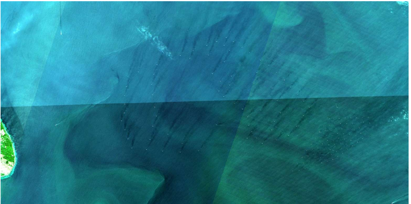
Figure 6: effects of windfarms on the roughness of surface and on turbulences in the atmosphere. The images shows regular pattern behind (lee) of the wind farm piles. If the effect is within the atmosphere or on the water surface, further investigation is needed. No influence seems to be on the water constituents.
